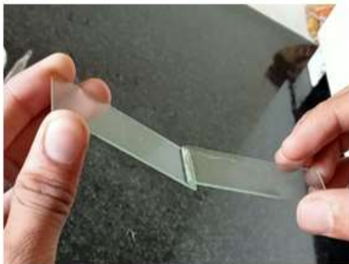
Figure 9: Spreadability testing using glass slides
