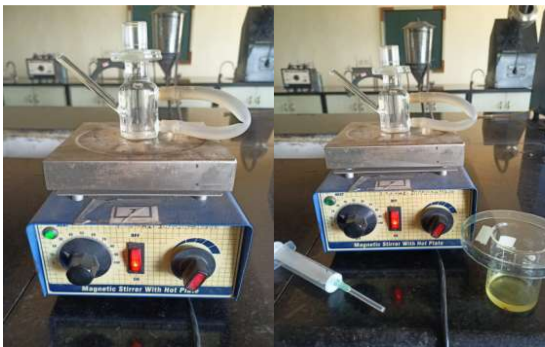
Figure. 14: Set up of Franz diffusion
