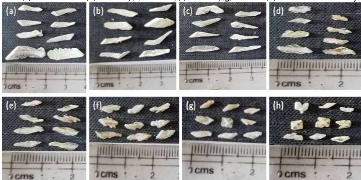
Figure 3: Scale measurement of harvested of struvite crystals(a) with magnesium acetate (b) with distilled water (c) with methanol (d) with 1%, (e) with 2%, (f) with 3%, (g) with 4% (h) with 5% after 15 th days.
