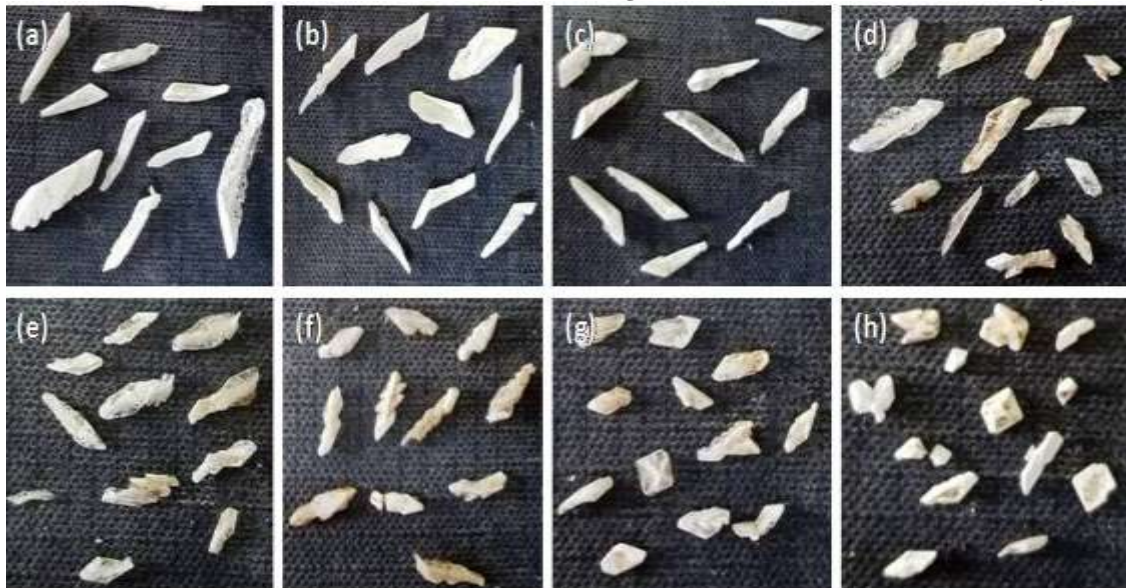
Figure 2: The harvested struvite crystals (a) with magnesium acetate (b) with distilled water (c) with methanol (d) with 1%, (e) with 2%, (f) with 3%, (g) with 4% (h) with 5% after 15 th days.
