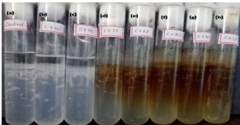
FIGURE 1: The effect of sample Snanoparticles on struvite crystals (a) with magnesium acetate (b) with distilled water (c) with methanol (d) with 1%, (e) with 2%, (f) with 3%, (g) with 4% (h) with 5% after 15 th days.
