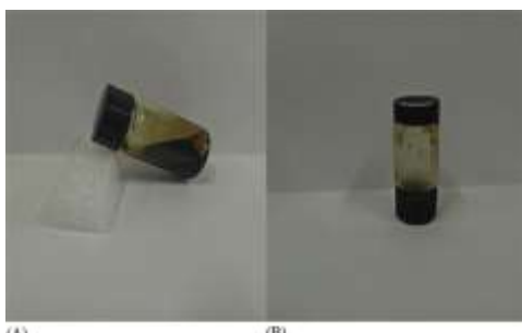
Fig 21. Thermal reversible property of the hydrogel. (A) the hydrogel was heated, (B) the hydrogel was cooled to room temperature.[23]
