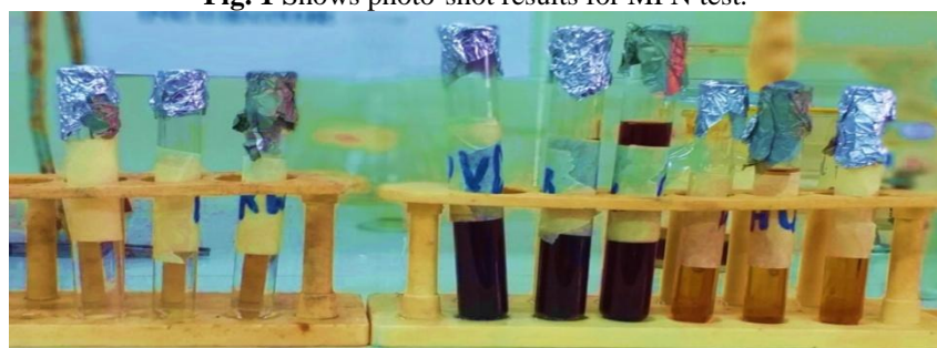
Sample preparation for MPN test ( 10\text{cm}^3 , 0.1\text{cm}^3 and 0.001\text{cm}^3 )
