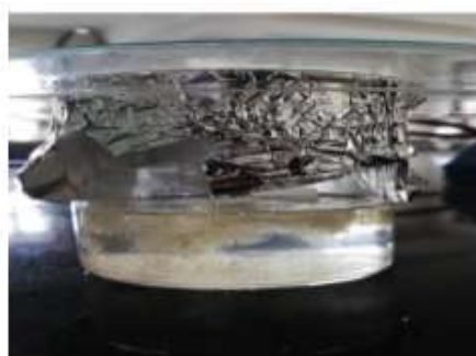
Figure 1: Swelling of polymer in water
