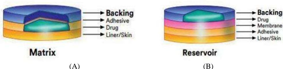
Fig.(A) Matrix And(B) Reservoir Type of Patches
