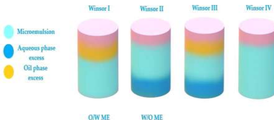
Fig 3. Winsor phases I, II, III, and IV are shown schematically to show how the phases change from Winsor phase I to Winsor phase IV to produce an ideal system.
