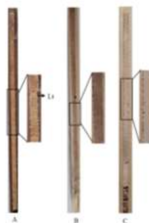
Figure 1. Wood cores (A) Pinusmerkusii; (B) Casuarina angustifolia; (C) Araucaria heterophylla. Lt. Latewood (growth ring)
