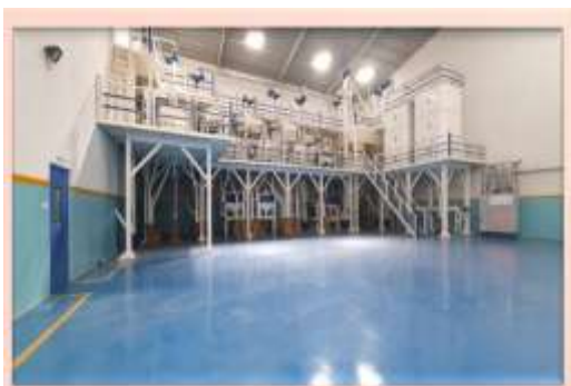
Cleaning Section (Set Of Different Sizes Of Sieves For Separating Different Materials From Seeds)
