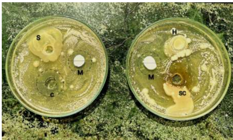
Figure 8: Zone of inhibition of different gels and marketed formulation (M- Marketed formulation, C - Carbopol, S - Sodium alginate, H - HPMC, SC - Sodium CMC)
