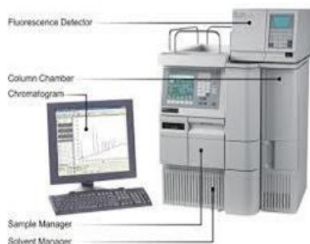
FIGURE NO: -1 WORKING DIAGRAM OF HPLC
