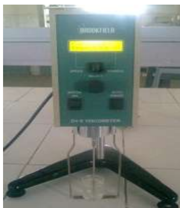
Figure2: Viscosity measurement by Brookfield viscometer
