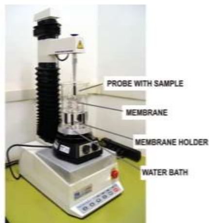
Fig: Bioadhesion test using the texture analyzer
